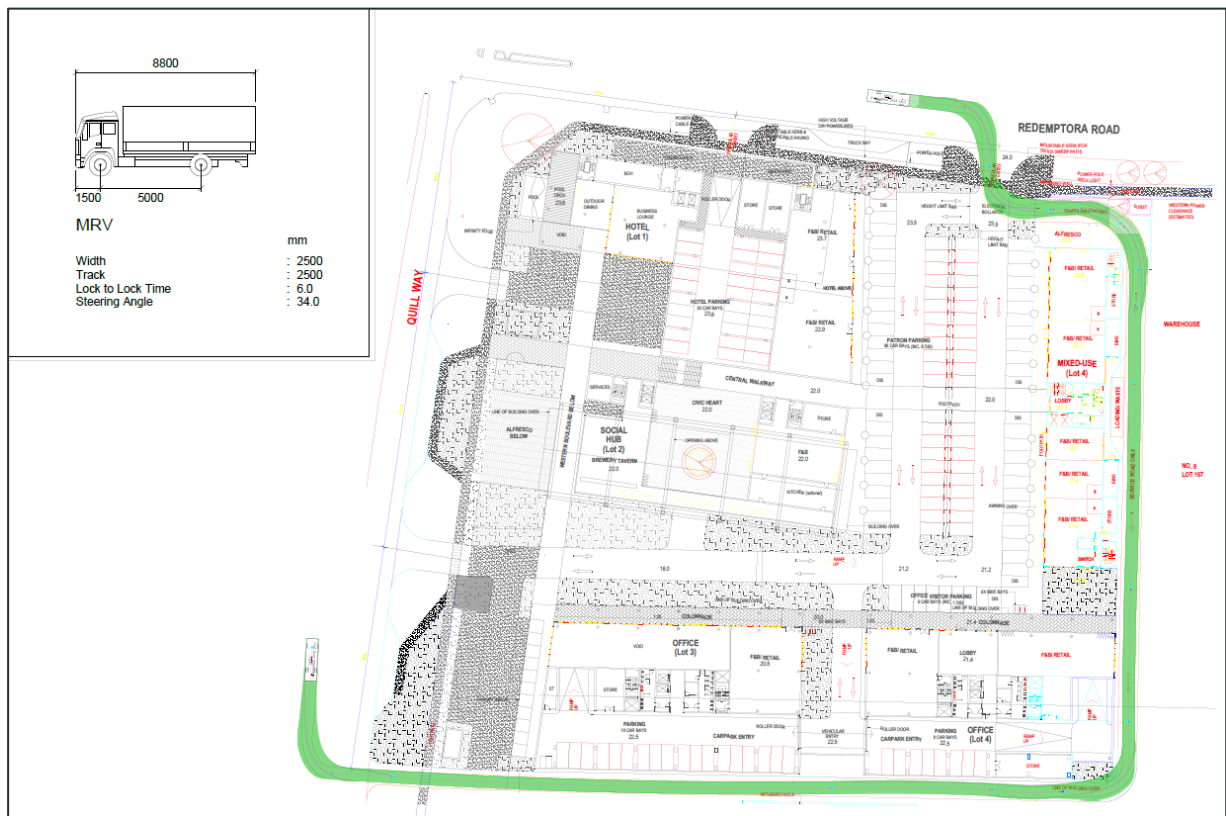
Figure 16 MRV Swept Path for Site Circulation
