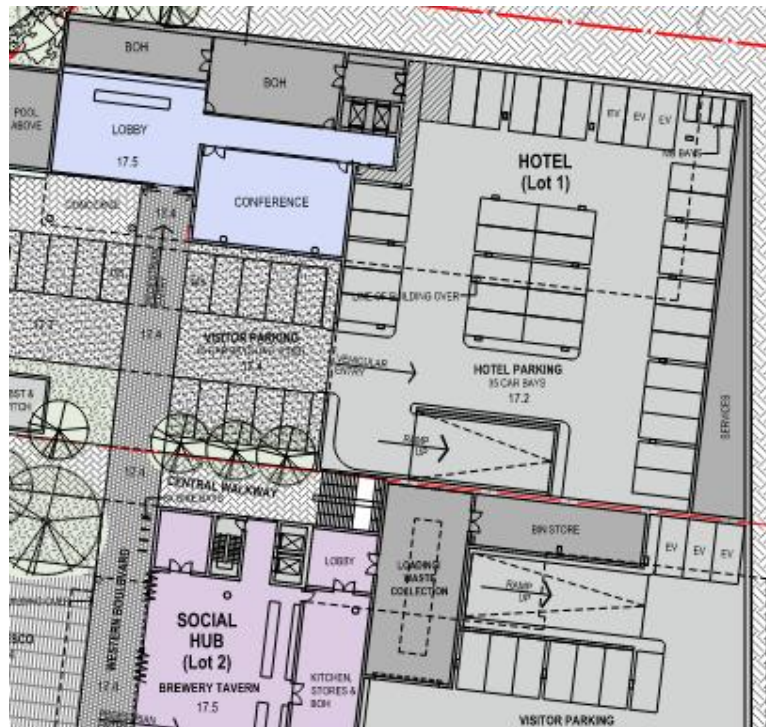
Figure 4: EV charging bays on Level B
