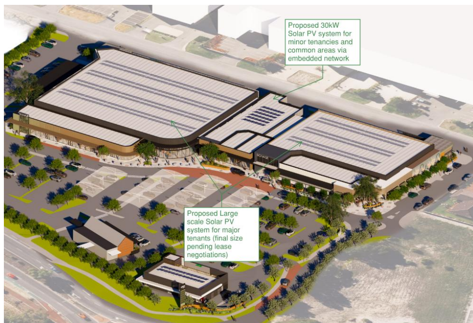
Figure 2 – Allocated Roof Area for Solar PV
